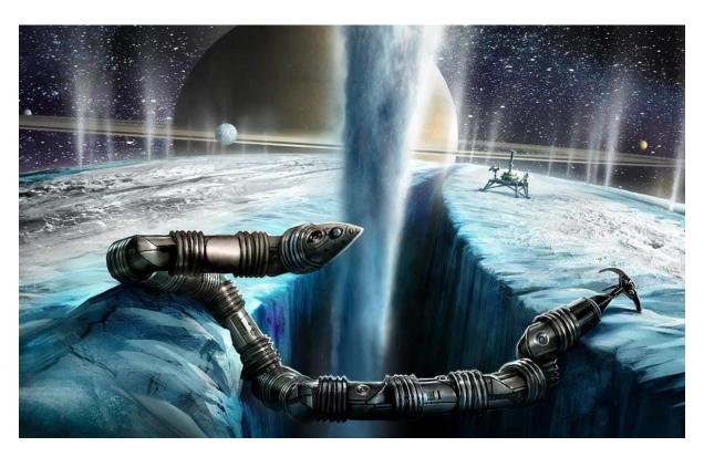
Using stereo cameras and lidar, EELS is able to create a 3D map of its surroundings, understanding the environment before navigating through it. JPL engineers have designed the robot to be able to independently slither through a variety of planetary and lunar terrains—from undulating sand and ice to steep cliffs, gaping craters, underground lava tubes and even narrow spaces within glaciers.
